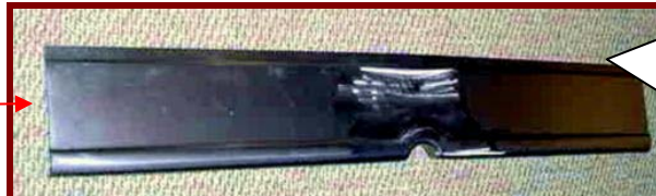
Lower Outer Rear Reveal – As Original Replaces the Bottom 5" of the Rear of the Cab up to 1 Ton
