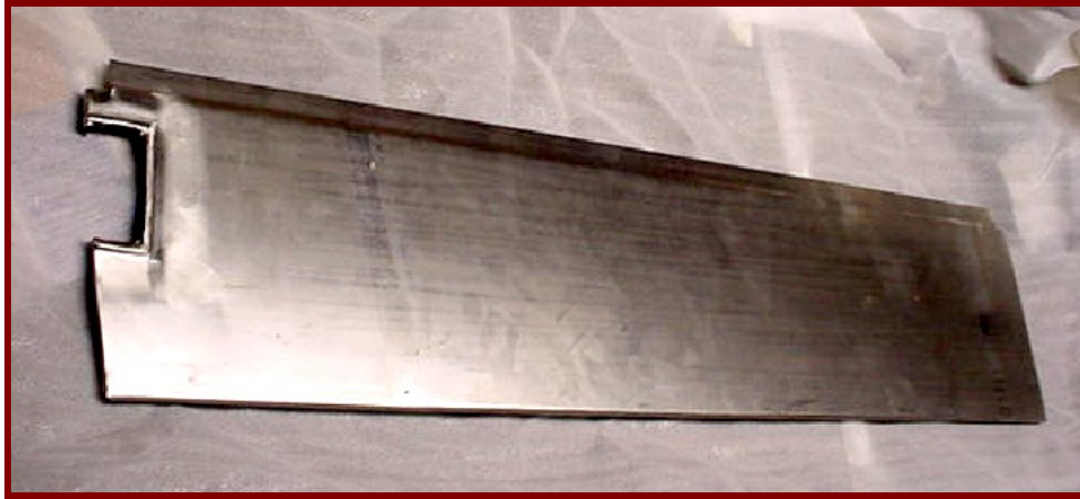
Lower Door Outer Repair Panel
